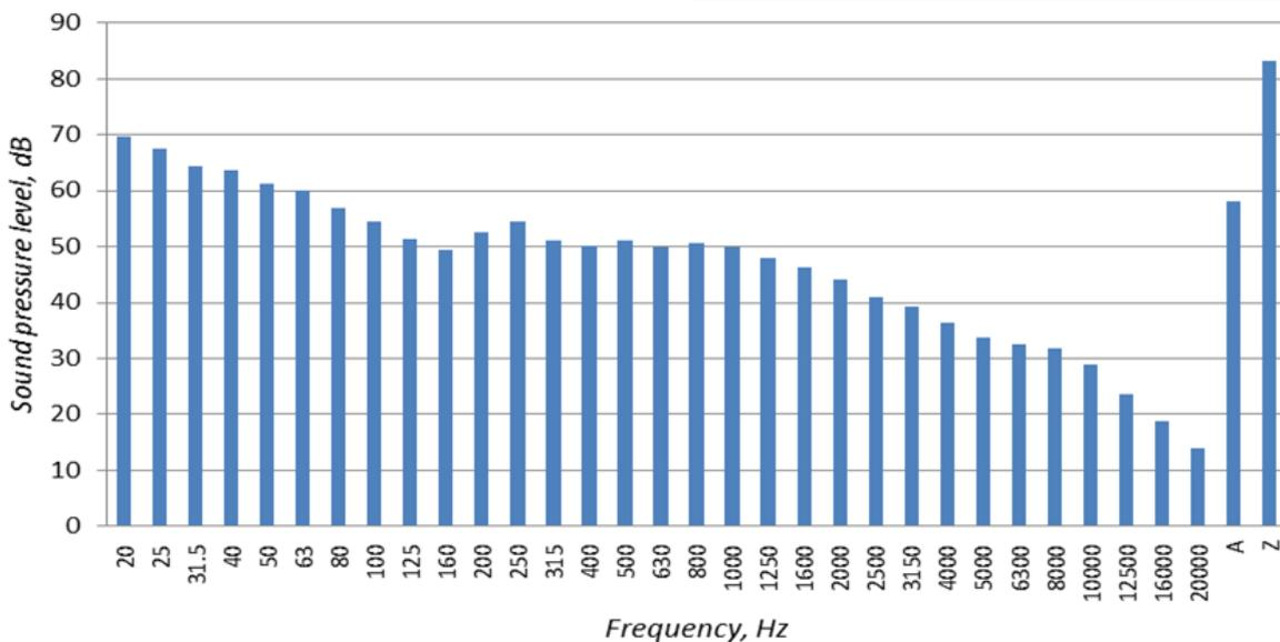
Figure 4 The noise spectrum of heat exchanger station
