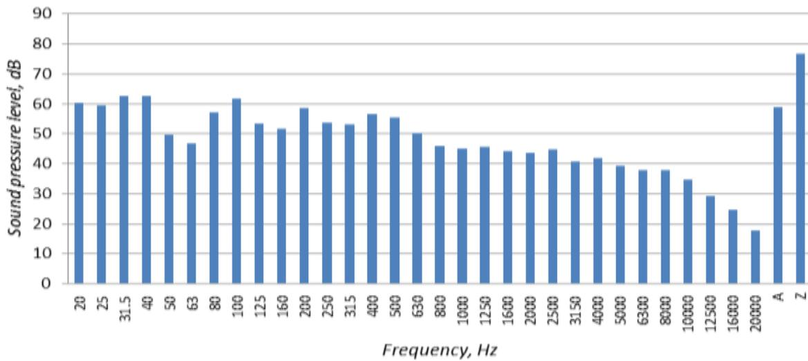
Figure 3 The noise spectrum of the transformer station
