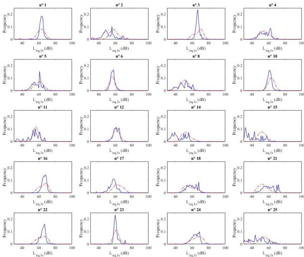
Figure 2. Sound level distributions ( $L_{eq,ls}$  in dB), from simulations (line, blue) and measurements (dots, red), for each of the 21 stations.
