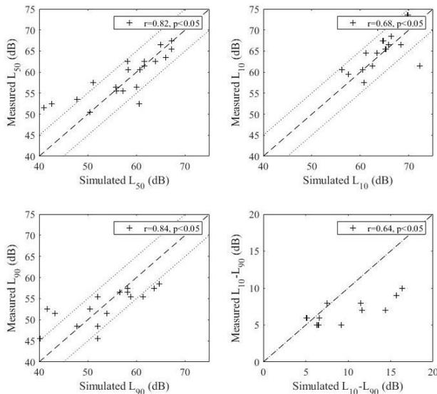
Figure 3 Comparisons between measured (vertical axis) and simulated (horizontal axis) statistical sound level indicators ( $L_{50}$ ,  $L_{10}$ ,  $L_{90}$ ,  $L_{10}$ - $L_{90}$ ) in dB.
