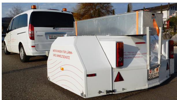
Figure 1: Modified CPX trailer to apply the required weight according to the tyre's load index.
