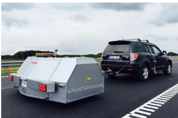
Figure 2 CPX measurement equipment
