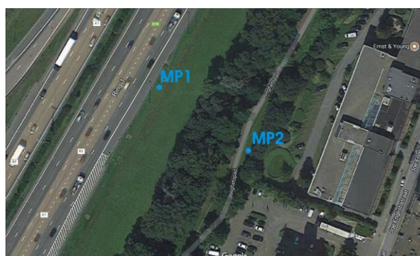
Figure 1. Positioning of microphones at MP1 and MP2 near part of the highway under study. MP2 is positioned on an embankment.
