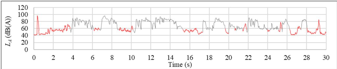
Figure 2 Example of a sound sample with indication of analyzed signal (gray) and silent and/or unwanted sounds in a speech recording (red).
