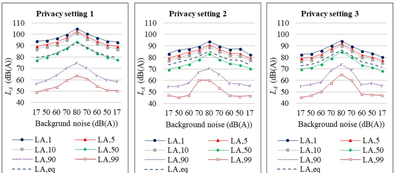
Figure 7 Statistical analysis of vocal effort and calculation of equivalent level of vocal effort depending on the background noise level.
