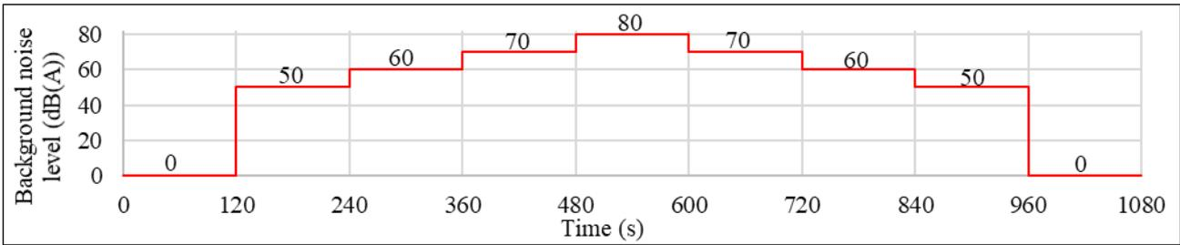
Figure 1 Profile of a background noise level, used during perception tests
