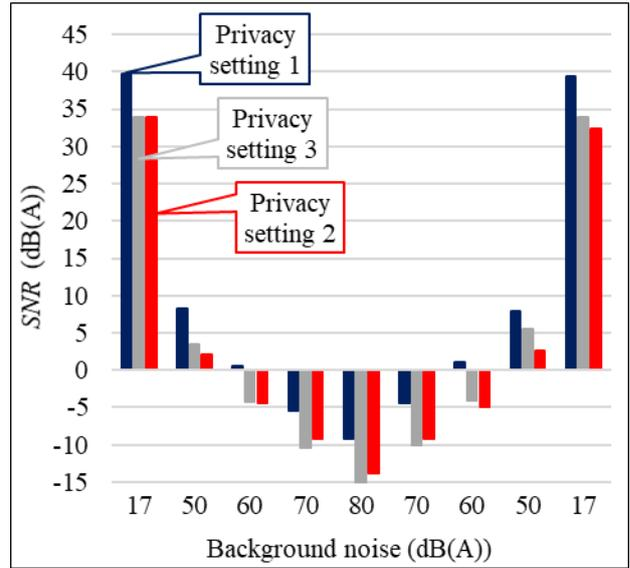
Figure 8 The signal-to-noise ratio at the position of listener at the variable distance.
