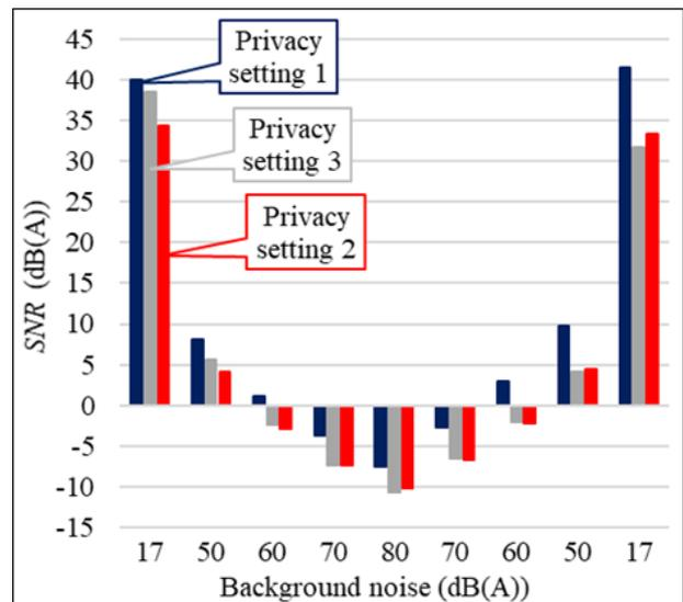
Figure 3 The signal-to-noise ratio at the position of listener at the distance 80 cm.
