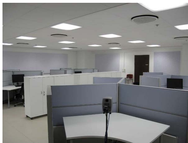
Figure 1. Top) The floor layout of the office. Speech was produced from loudspeakers of the corner workstations. Bottom) The ceiling drawing showing the positions of 18 sound masking speakers (red triangles) above the suspended ceiling, six ventilation inlet supplies (blue lines), and 16 luminaires (red crossed circles). Bottom) A photograph of the open-plan office. One of the corner loudspeakers is shown in front.
