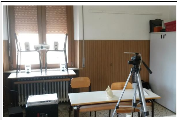
Figure 2. Positioning of the electro-acoustic system and of the measurement microphone in a classroom.
