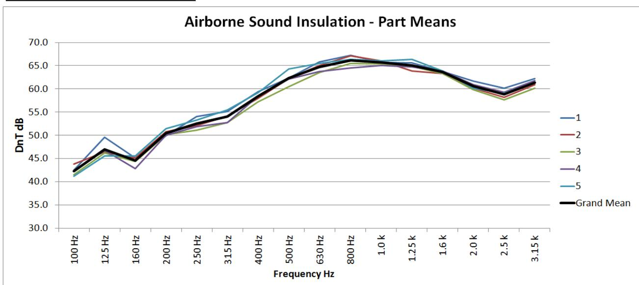
Figure 3: DnT means for each floor tested and grand mean of all floors
