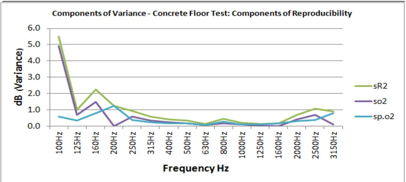
Figure 5: Variance components of Reproducibility (Operator + Operator by part interaction).
