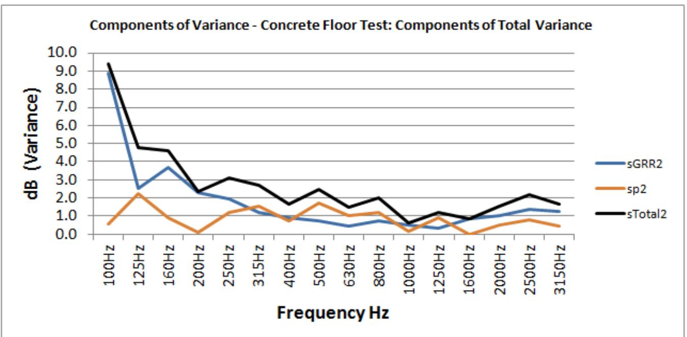
Figure 6: Total variance components (Gauge + Part to part)
