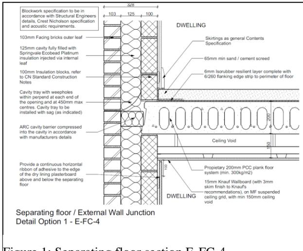
Figure 1: Separating floor section E-FC-4
