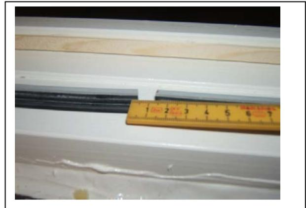
Figure 2. Picture of window N from test A with 10 mm opening in the sealing gasket.
