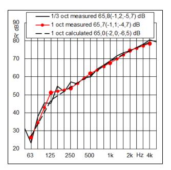
Figure 2. Curves and R' rated values of airborne sound pressure level in one-third and octave bands.
