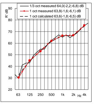
Figure 3. Curves and R' rated values of airborne sound pressure level in one-third and octave bands
