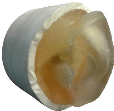
Figure 3. Example of outer ear experimental phantom fabricated from polymeric materials (© True Phantom)
