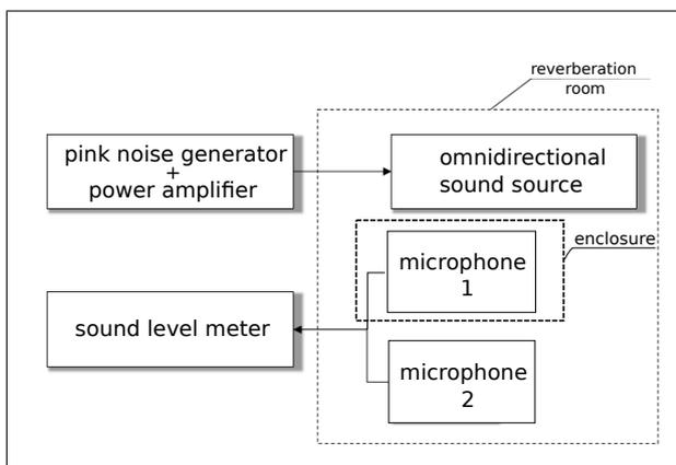
Figure 2. Reciprocity (RM) measurement method
