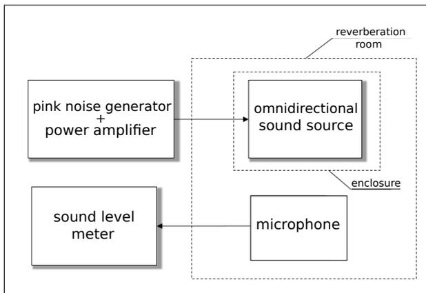
Figure 1. Actual source (AS) measurement method
