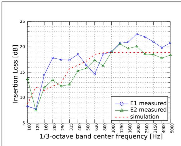
Figure 6. Insertion Loss of enclosures with different volumes (different modal overlaps). Enclosure E2 contains more modes in each frequency band. The graph refers to enclosures with light mineral wool and an leak ratio equal to 1 %, measuring method: RM
