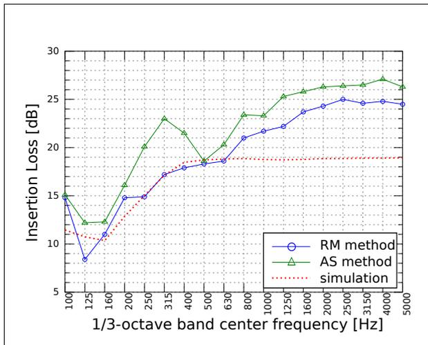
Figure 7. Insertion Loss of enclosures measured with different methods. The graph refers to enclosures with dense mineral wool and an leak ratio equal to 1 %, enclosure E2. The lack of convergence of measurements and simulations above 630 Hz has been explained in section 4.1.
