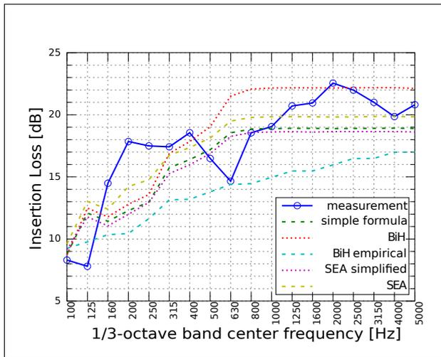
Figure 3. Insertion loss of enclosures obtained by using different models
