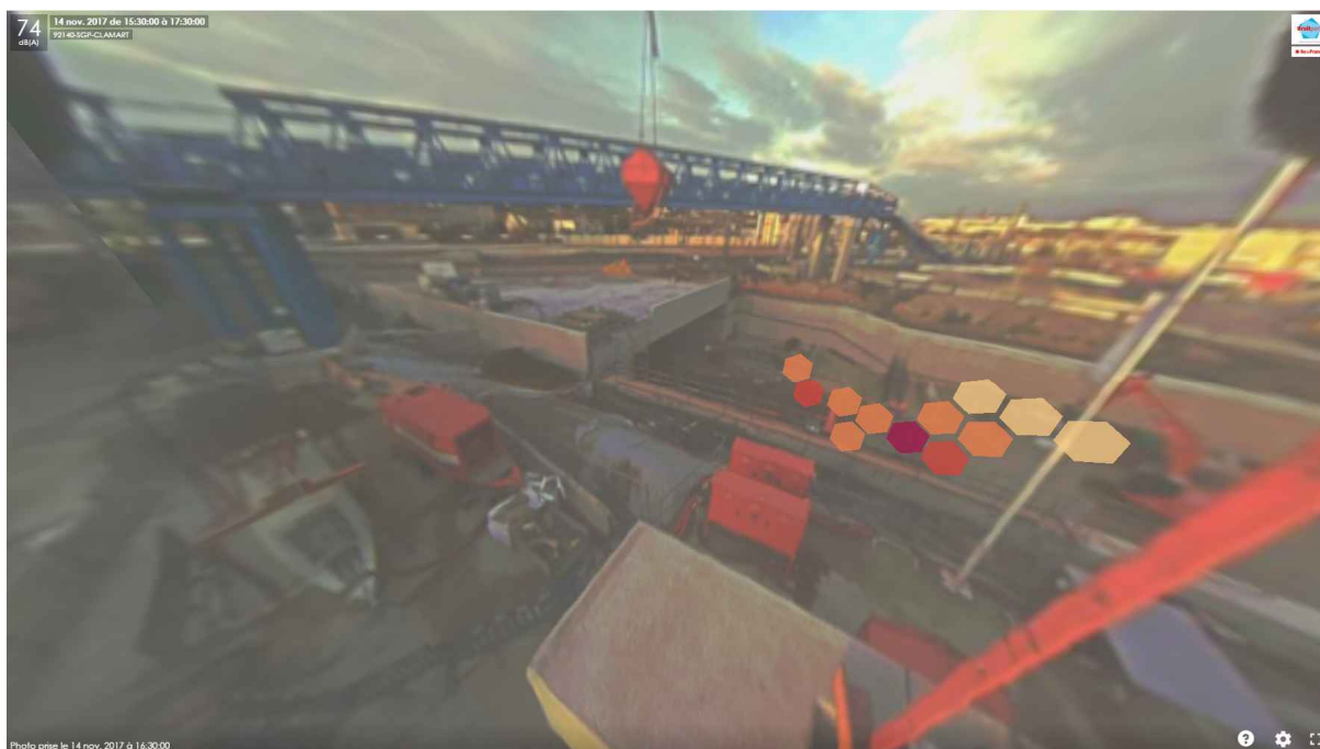
Figure 2: One of the images from one of the "medusa" sensor deployed at the Grand Paris Express construction site in Clamart. It shows that two thirds of the sound energy emitted towards this sensor, during two hours between 15h30 and 17h30 on November 14, 2017, comes from a precise place of the construction site (in red). The noise level observed at the sensor is 74 dB(A).
