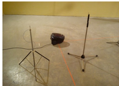
Figure 10. Measurement of the vacuum cleaner in the reverberant room.
