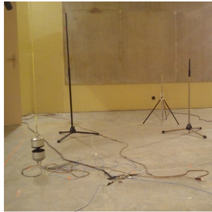
Figure 6. Sound power measurement set-up in a large reverberation room.
