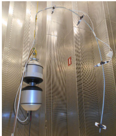
Figure 5. Free-field measurement set-up for sound power and directionality
