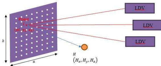
Figure 3. Method based on the linear superposition of effects – estimation of the sound pressure level in front of the vibrating surface.
