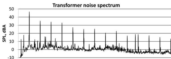
Figure 1. Transformer noise spectrum at load conditions.
