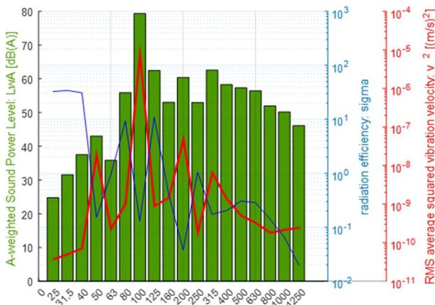
Figure 4. Radiation efficiency vs A-weighted sound power level vs RMS average squared vibration velocity.
