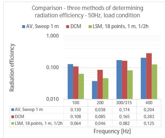
Figure 5. Comparison of three methods of determining radiation efficiency – 50 Hz, load condition.
