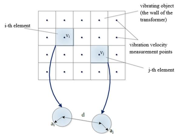
Figure 2. The idea of Discrete Calculation Method.
