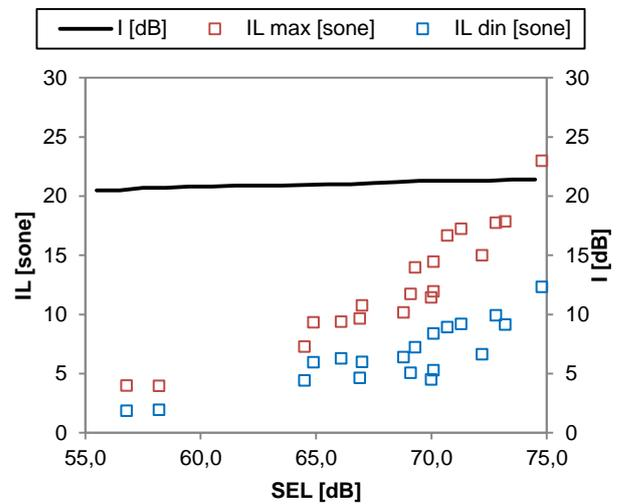
Figure 2. Graphical comparison between impulsiveness and loudness-based impulsiveness obtained for train cars collisions with  $SEL$  value range 56.8 – 78.8 dB.
