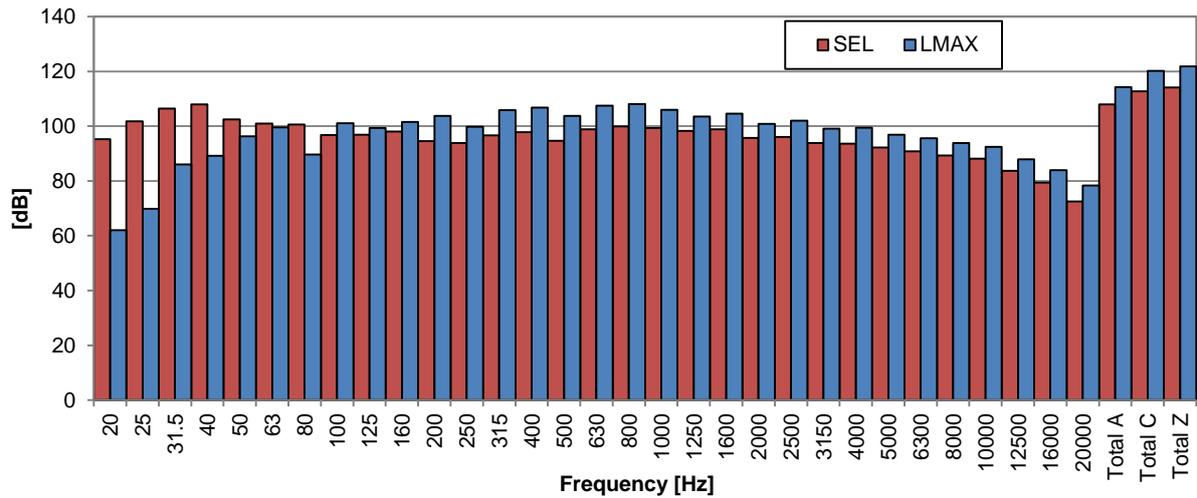
Figure 1. SEL spectrum and maximum level spectrum of collision of wagons registered close to the noise source.
