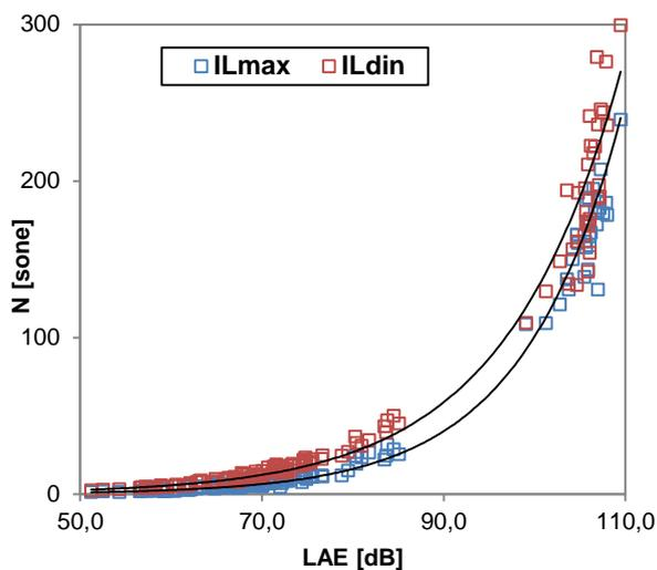
Figure 3. Instantaneous Loudness-based impulsiveness  $IL_{max}$ ,  $IL_{din}$  as a function of sound exposure level.
