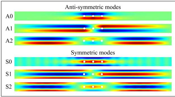
Figure 4. The first three orders of eigenmodes associated with the edges of the narrow gap at the  $\Gamma$  point  $qd/\pi = 0$ . The symmetric and anti-symmetric modes are categorized according to their symmetry with respect to the  $x$ -axis. From top to bottom, the eigenfrequencies (in Hz) are 15125 (A0), 15414+0.5i (A1), 15472+3.1i (A2), 15257+13.2i (S0), 15441+1.9i (S1) and 15478+6.0i (S2), respectively. Note that the eigenfrequencies slightly increase with the order of the guided modes.
