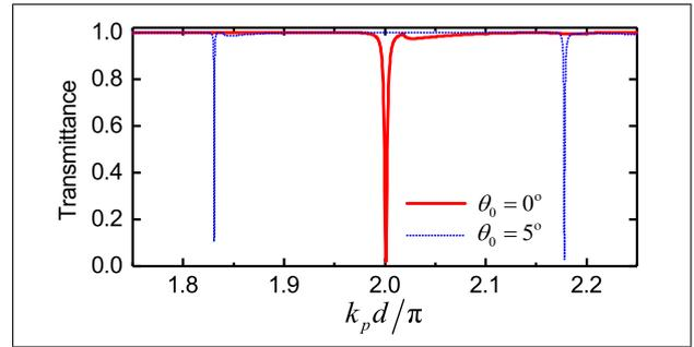
Figure 5. Transmittance spectra obtained when a plane wave impinges on an infinite platonic crystal slab consisting of three layers of free holes. The solid and dotted lines represent the results in cases  $\theta_0 = 0^\circ$  and  $\theta_0 = 5^\circ$ , respectively. From left to right, the frequencies of the three minimums are 1.83, 1.99 and 2.18 (in reduced units), respectively.
