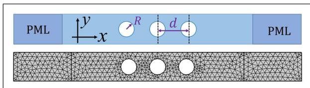
Figure 1. Numerical model of an infinite platonic crystal slab consisting of three layers of free holes.
