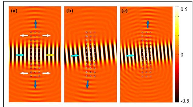
Figure 6. Multiple scattering simulations showing the interaction of a Gaussian beam impinging on a platonic crystal slab. From left to right, the impinging frequencies are 15.40 (a), 13.02 (b) and 18.43 kHz (c), corresponding to the frequencies of the three minimums observed in Figure 5. The arrows indicate the main energy fluxes.
