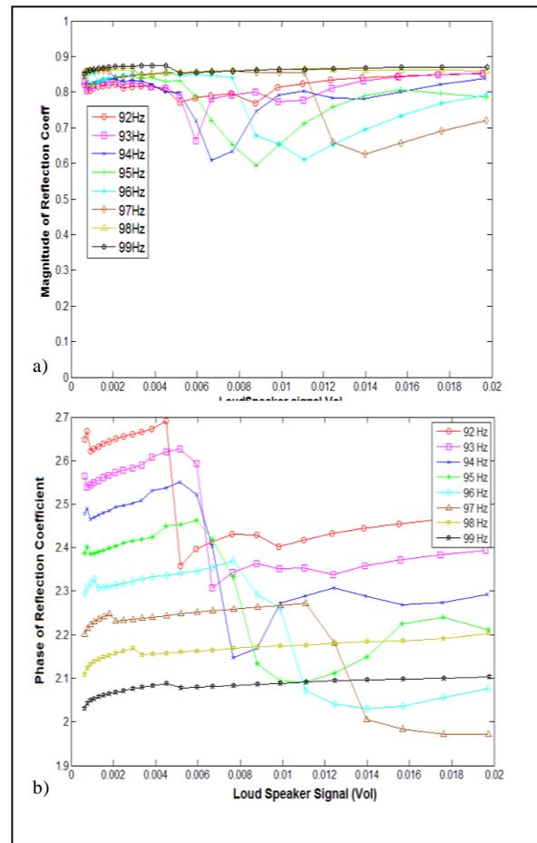
Figure 9. Effect of NET in BC3 on teflection coefficient. a) Magnitude; b) Phase.
