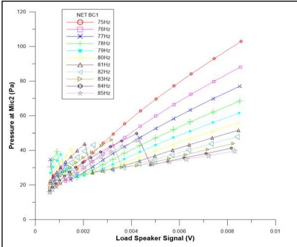
Figure 4. Pressure amplitude at the midsection of the duct (Mic.2) showing the occurrence of NET (BC1).
