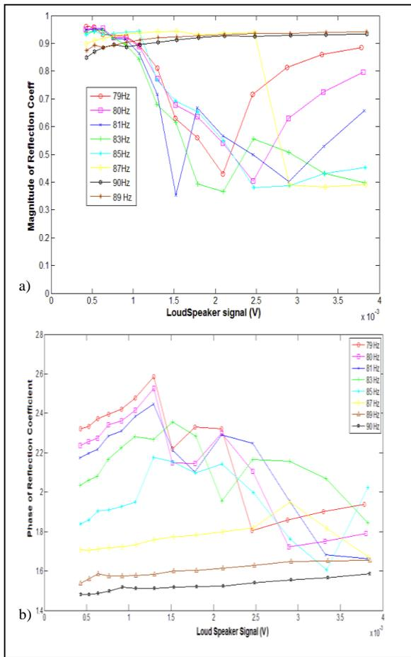
Figure 7. Effect of NET in BC2 on teflection coefficient. a) Magnitude; b) Phase.
