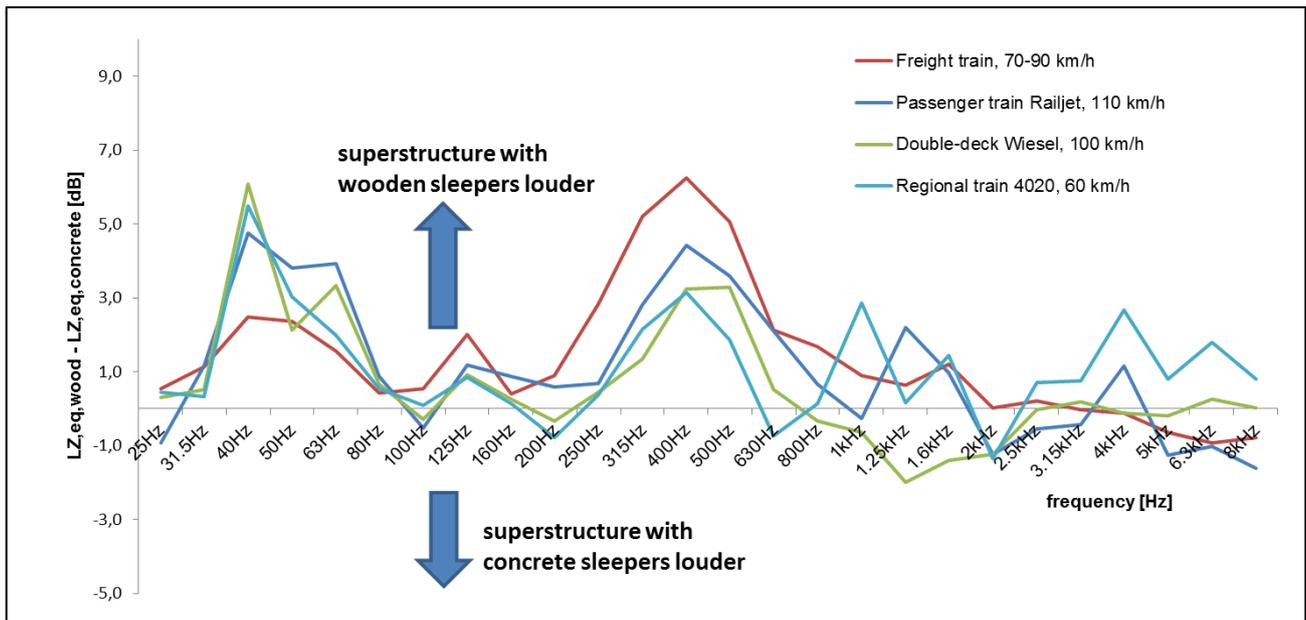
Figure 3. Difference of the emissions on wooden sleepers compared to the emissions on concrete sleepers.
