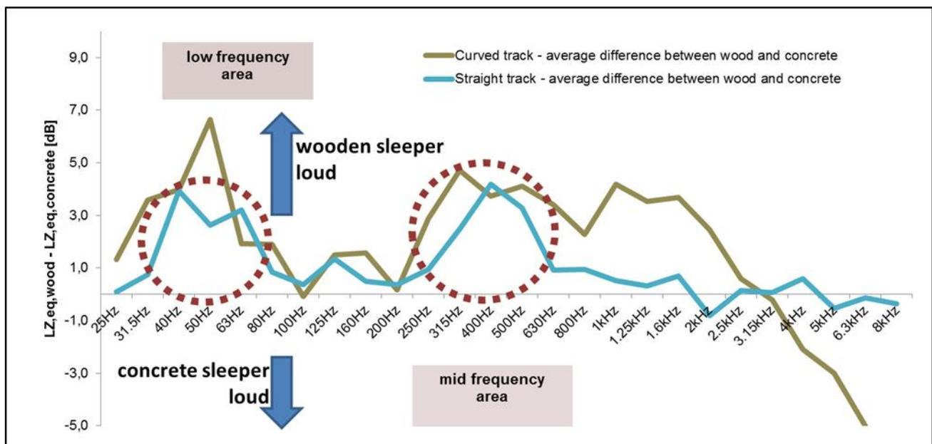
Figure 4. Difference of the emissions between wooden and concrete sleepers for the straight and the curved track averaged over all train types.
