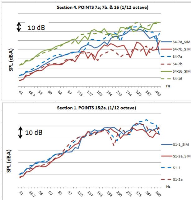
Figure 8. Wall pressure spectral results for S1 & S4 (for positions see sketch in Figure 7)
