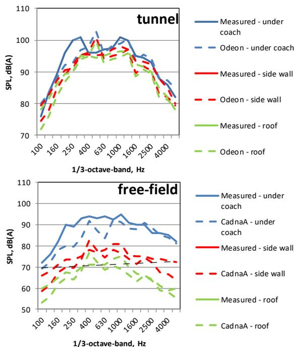
Figure 15. Measured and calculated 1/3 octave band SPL on carbody surface areas in dB(A) (top: tunnel, bottom: free field).
