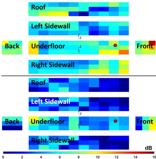
Figure 4. Geometry influence (SPL difference) calculated with BEM. Top: 100 Hz, Bottom: 1000 Hz
