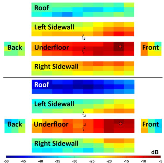
Figure 3. BEM calculated TF (SPL – SWL) for source at left front wheel/rail contact. Detailed geometry. Top: 100 Hz, Bottom: 1000 Hz
