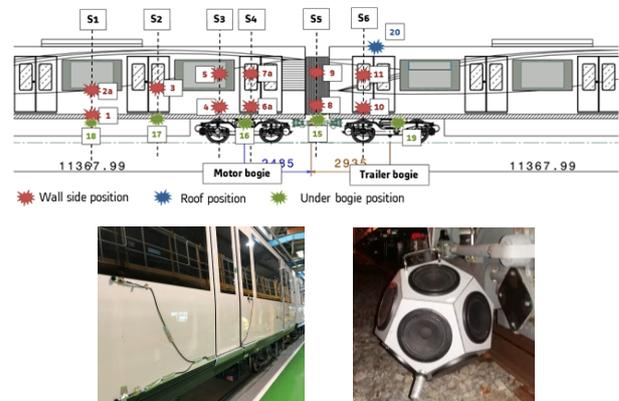
Figure 5. Metro at standstill - measurement set-up with omnidirectional loudspeaker beside the bogie.
