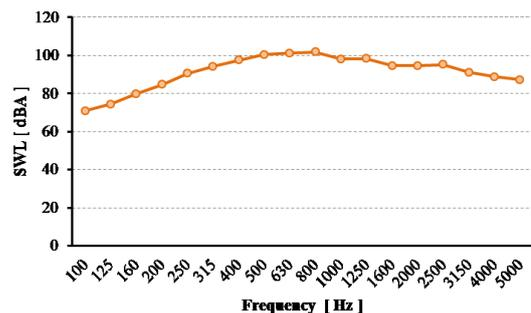
Figure 10. Rolling noise SWL spectrum of a metro wheelset running at 80 km/h.
