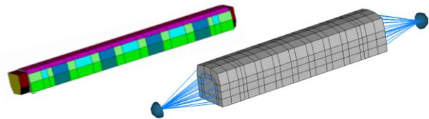
Figure 9. VAOne model of a metro trailer coach (left) and exterior acoustic cavities (right)
