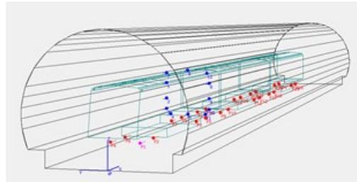
Figure 13. Geometric layout of input data (tunnel shape, carbody with three cars, red dots: sound source for each wheel; blue dots: receiver positions).
