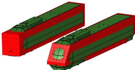
Figure 1. Simplified (left) and more detailed (right) meshed geometry of carbody in red in comparison to real train geometry (in green)
