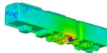
Figure 6. Metro BEM model including source location and overall SPL distribution (40-500 Hz).
