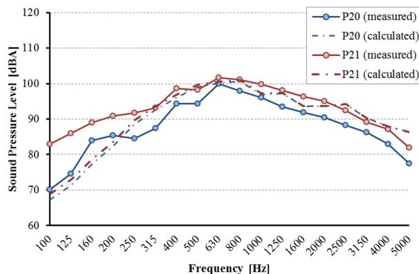
Figure 12. Measured vs. calculated wall pressures at microphones 20 and 21.
