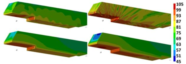
Figure 2. SPL distribution on carbody for source at right front wheel/rail contact at 100 and 1000 Hz (105 dB SWL per frequency assumed). Left: 100 Hz, Right: 1000 Hz. Top: BEM, Bottom: Ray acoustics
