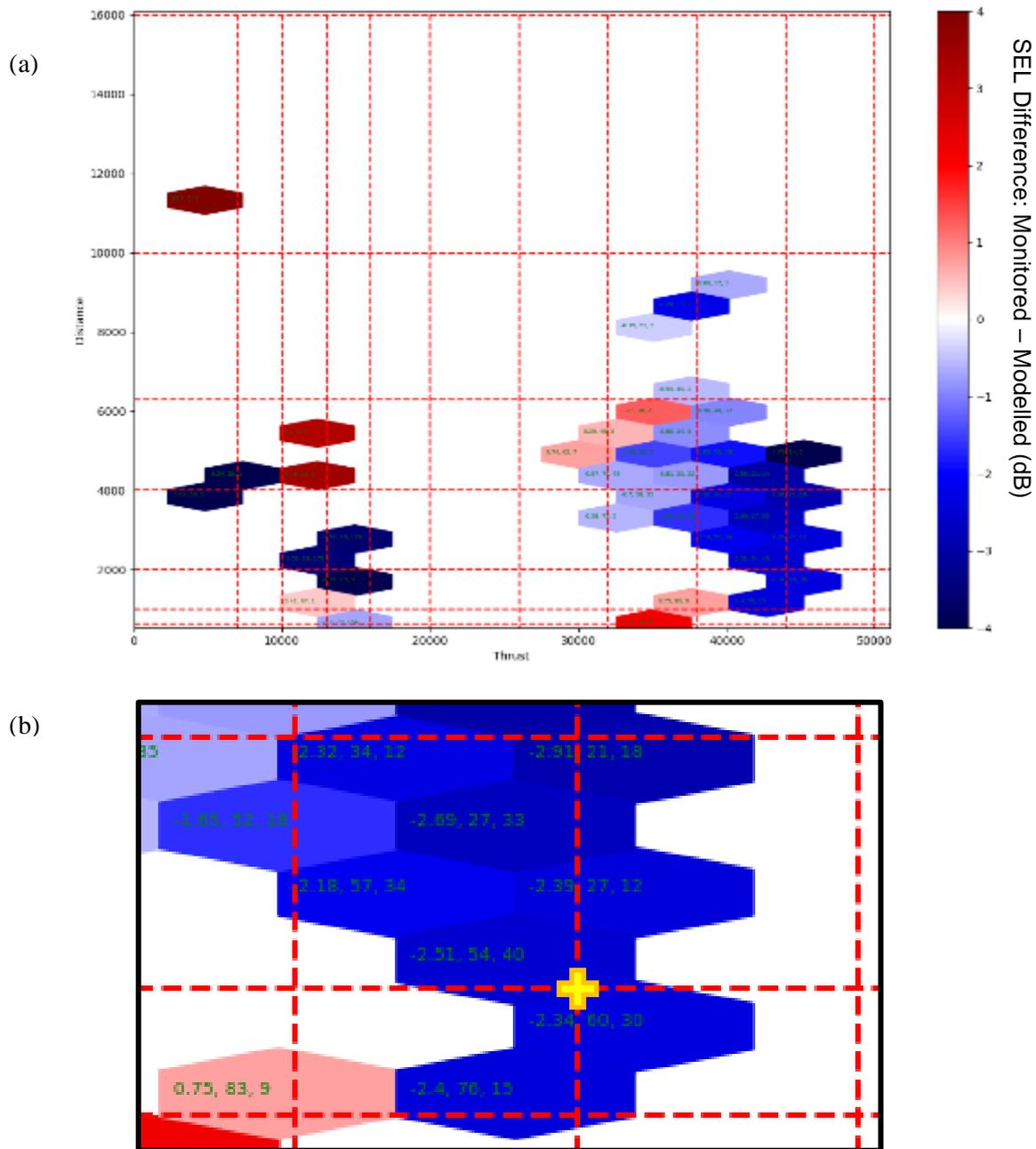
Figure 9 (a) Hexagon bin plot for the 747400 aircraft using the data designed profile and the original NPD curves. (b) Zoomed in section around the point (44000,2000).
