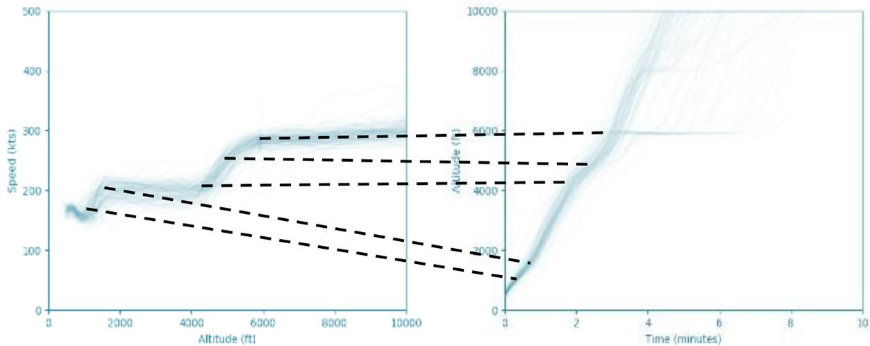
Figure 5. Example identifying procedure steps
