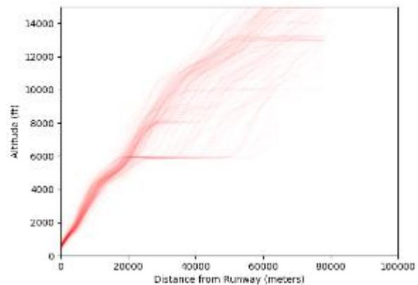
Figure 2. Aircraft altitude against track distance
