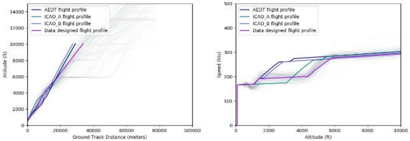
**Figure 7.** Example profiles for the 747400 stage 5 departure on 09R showing the profiles from the data in grey, the AEDT flight profile in navy and the profile designed from data in purple. The data designed profile has a much better fit
