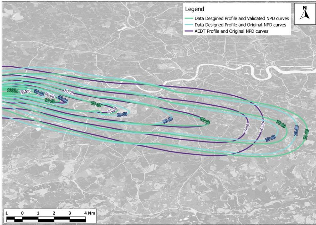
Figure 12 Noise contours for the 747400 stage 5 departure on the 09R DET route for a single flight. Contours are shown for the three scenarios which have been used in the examples above. All three scenarios use the same track, but the flight profile and NPD curve are altered as described in the figure legend.
