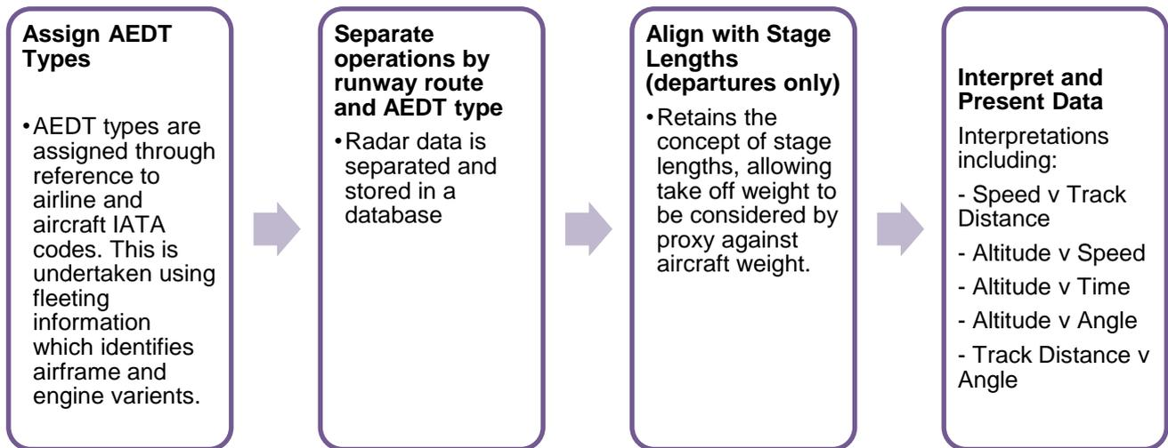
Figure 4. Process steps for describing aircraft performance
