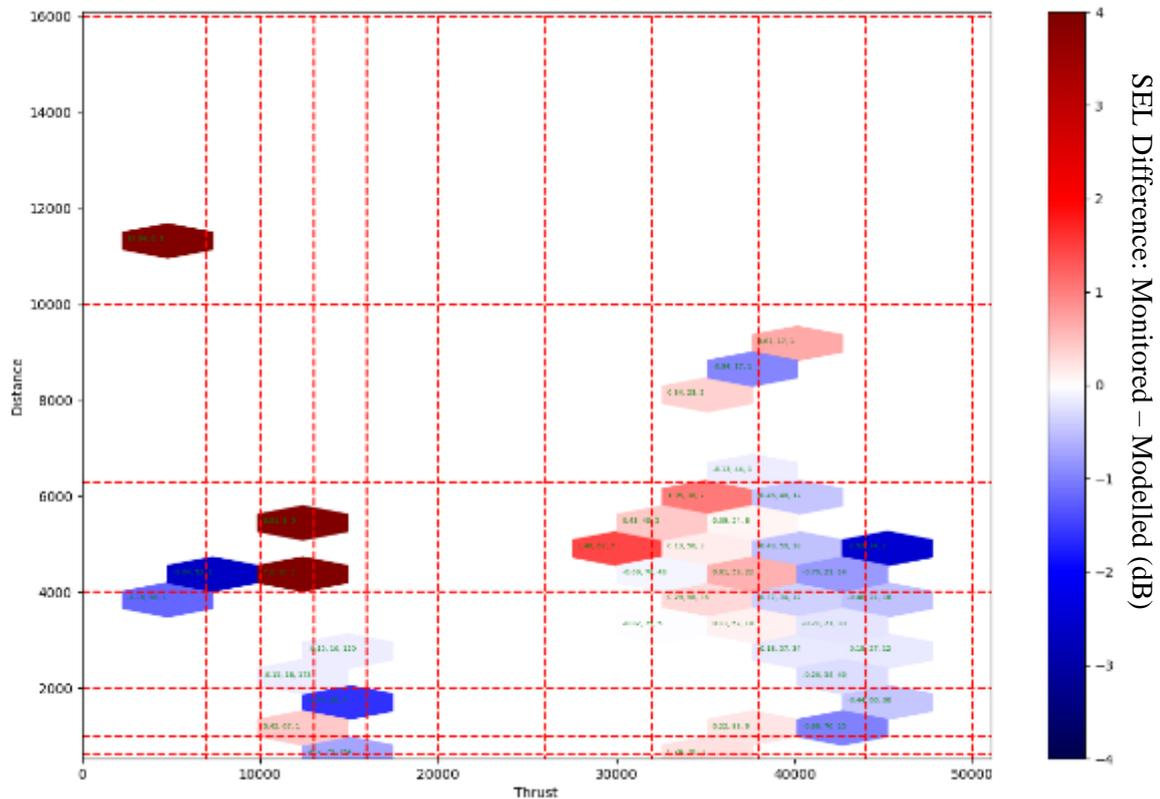
Figure 10 Hexagon bin plot for the 747400 aircraft using the data designed profile and the validated NPD curves. The differences in this plot are much smaller than those observed in Figure 9 (a).
