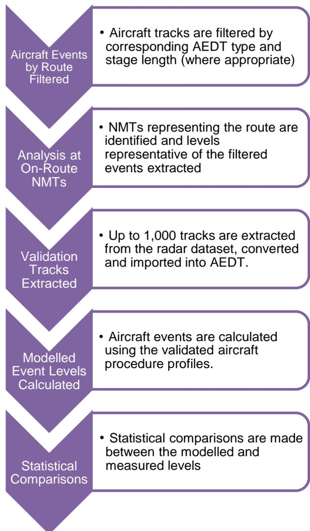
**Figure 8.** Staged process for obtaining noise event comparisons
