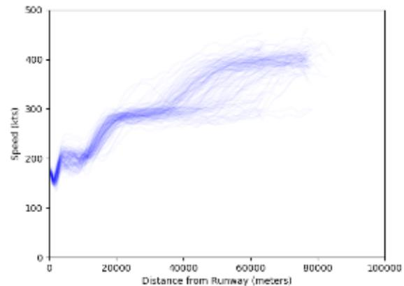
Figure 3. Aircraft speed against track distance
