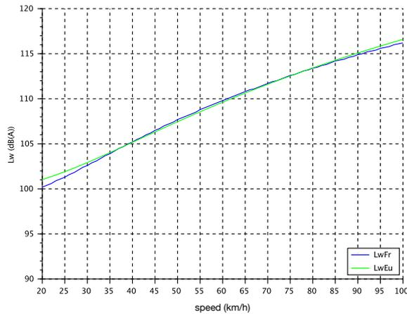
Figure 8. Best fit of the EU model against the FR model based on  $L_W$  for HGV and R3 Non drainage pavement.
