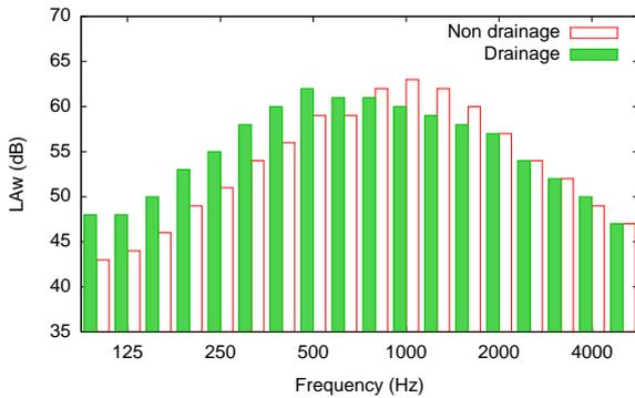
Figure 1. Fixed frequency distribution  $R_i$  for Drainage and Non drainage pavements.
