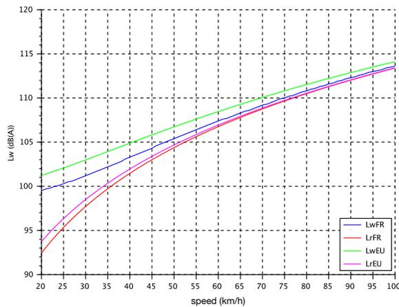
Figure 5. Best fit of the EU model against the FR model based on  $L_r$  for HGV and R1 Drainage pavement.
