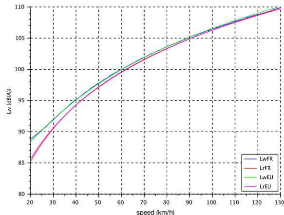
Figure 2. Best fit of the EU model against the FR model based on  $L_r$  for LV and R2 Non drainage pavement.
