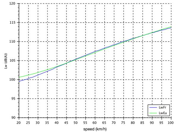
Figure 6. Best fit of the EU model against the FR model based on  $L_W$  for HGV and R1 Drainage pavement.
