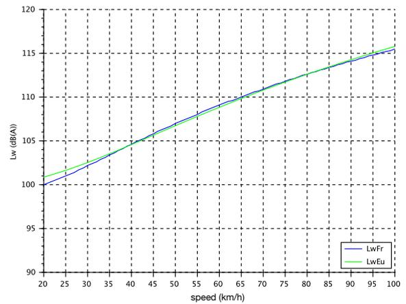
Figure 7. Best fit of the EU model against the FR model based on  $L_W$  for HGV and R2 Non drainage pavement.
