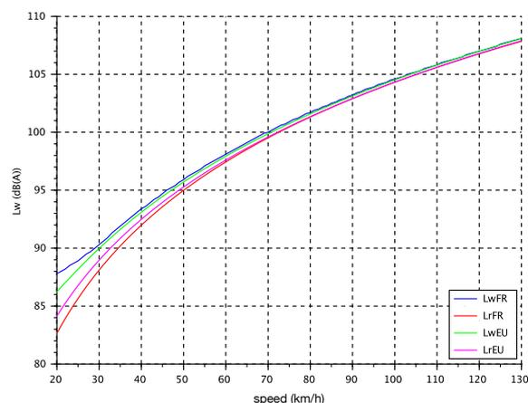
Figure 3. Best fit of the EU model against the FR model based on  $L_r$  for LV and R1 Non drainage pavement.
