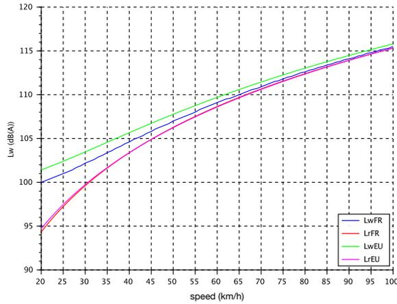
Figure 4. Best fit of the EU model against the FR model based on  $L_r$  for HGV and R2 Non drainage pavement.
