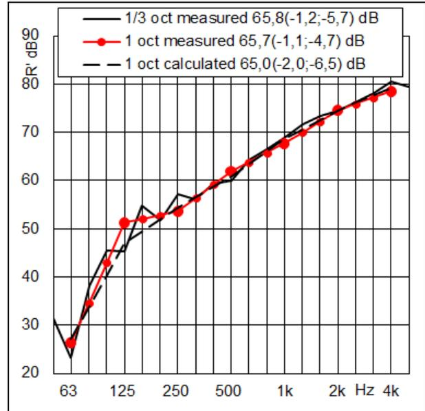
Figure 2. Curves and  $R'$  rated values of airborne sound pressure level in one-third and octave bands.
