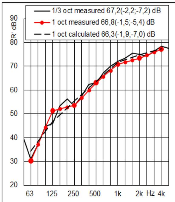
Figure 1. Curves and  $R'$  rated values of airborne sound pressure level in one-third and octave bands.
