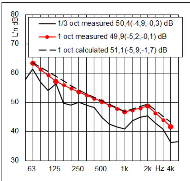
Figure 5. Curves and  $L'_n$  rated values of impact sound pressure level in one-third and octave bands.
