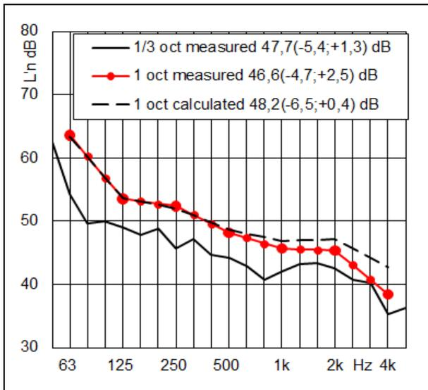
Figure 4. Curves and  $L'_n$  rated values of impact sound pressure level in one-third and octave bands.
