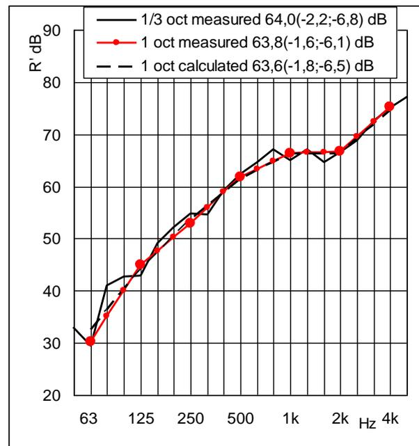
Figure 3. Curves and  $R'$  rated values of airborne sound pressure level in one-third and octave bands
