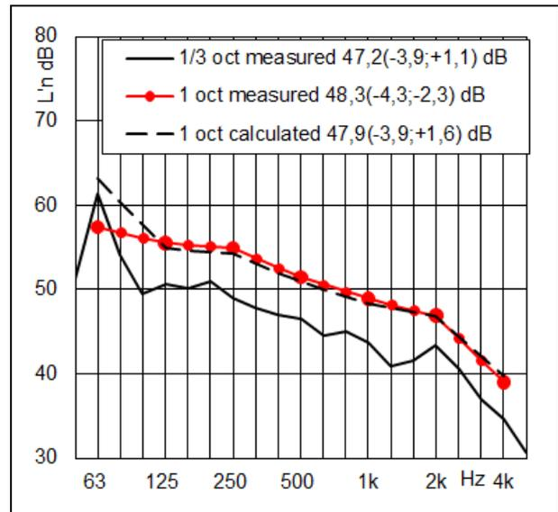
Figure 6. Curves and  $L'_n$  rated values of impact sound pressure level in one-third and octave bands.
