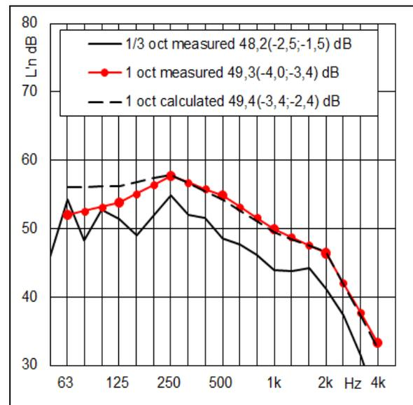
Figure 7. Curves and  $L'_n$  rated values of impact sound pressure level in one-third and octave bands.
