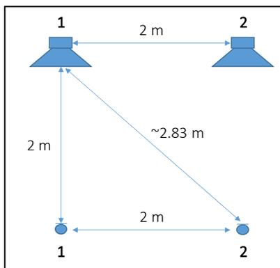
Figure 4. Test setup for ICA.
