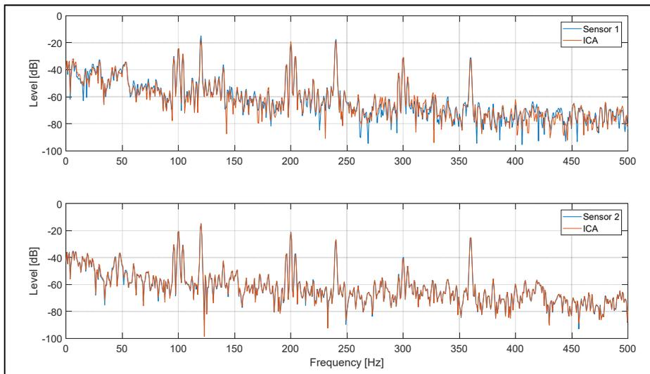
Figure 8. ICA test measurement results with loudspeakers and microphones.
