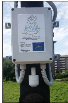
Figure 2: Smart-noise monitoring system
