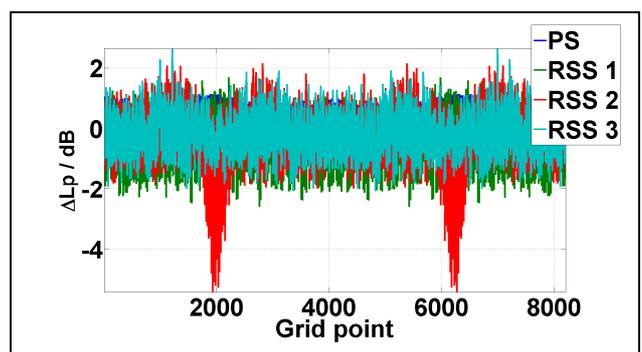
Figure 6. Sound pressure level difference between the originally measured sound pressure and the sound pressure using the spherical harmonics transform coefficients for each measurement grid point.
