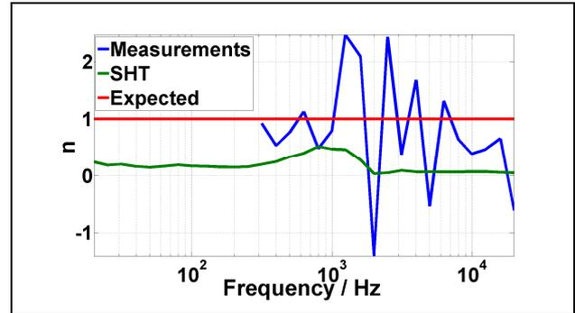
Figure 10. RSS spherical harmonics order after measurements, spherical harmonics transform and expected value against frequency.
