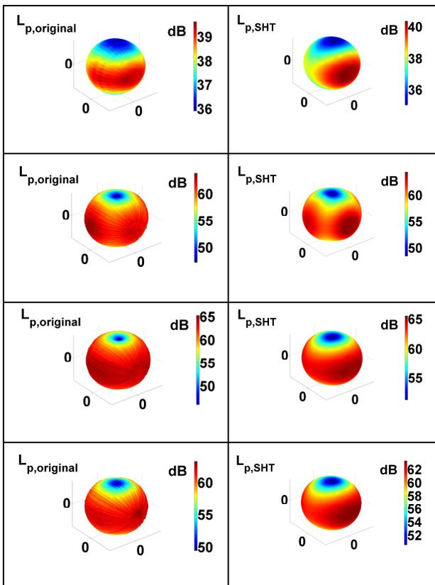
Figure 5. Sound pressure level over a sphere for the primary source (first row) and three reference sound sources (other rows) at 80 Hz. Left column: originally measured data. Right column: Data after spherical harmonics transform.
