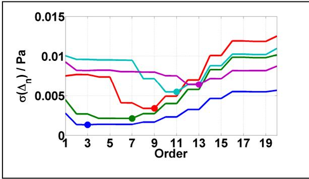
Figure 4. Determination of spherical harmonics order for five different 1/3 octave bands (different colours) for a reference sound source. The dots represent the selected order for each band.
