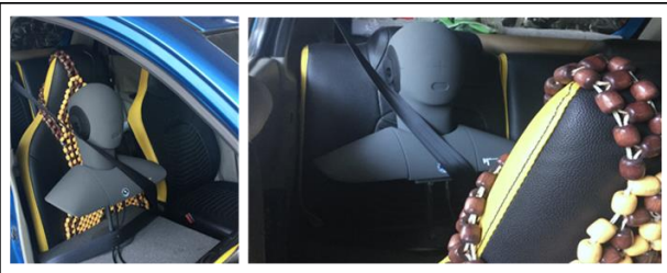
Figure 8. Cabin characteristics transfer function measurements using binaural responses at Driver Ear and Rear Passenger Ear locations
