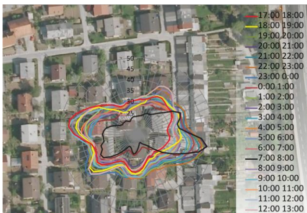
Figure 5. Immission directivity of noise at the ML in settlement near the highway, for different time intervals of the day.
