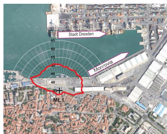
Figure 8. Noise immission directivity at ML1 indicates that traffic noise is dominant for given noise propagation conditions
