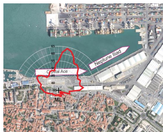
Figure 10. Noise immission directivity at ML1 indicates that at the middle of the closest ship is dominant noise source for given noise propagation conditions
