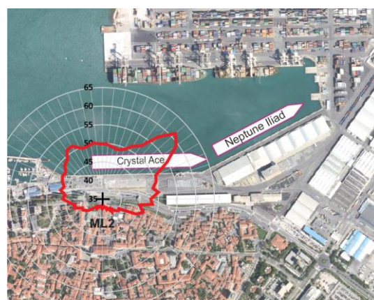
Figure 9. Noise immission directivity at ML2 indicates that at the middle of the closest ship is dominant noise source for given noise propagation conditions
